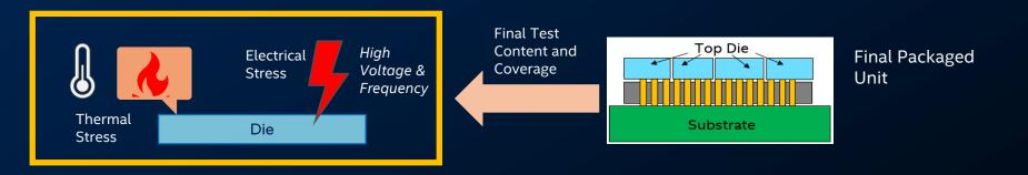
KGD = Passing Die under stress from all the test conditions
