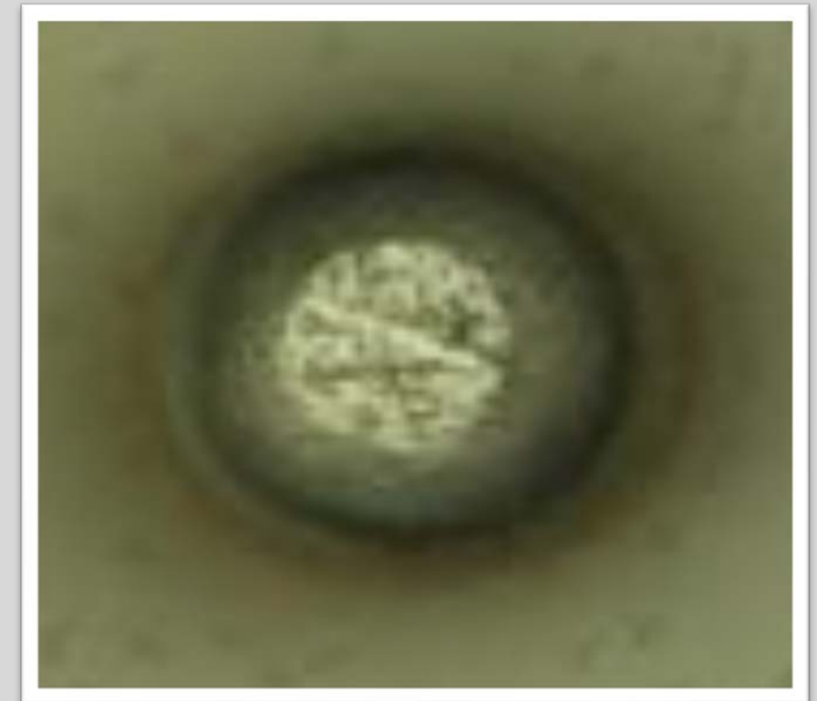
Bump mark of 1.7um depth and 16.7um circumference by MT80F
