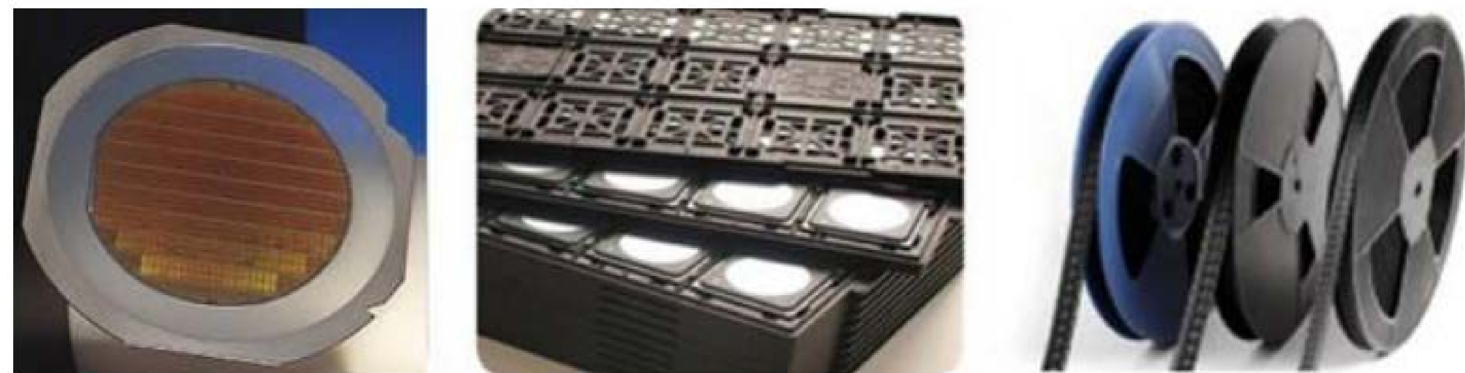
Fig. 1: Dicing film, JEDEC trays and Tape & Reel- commonly used device handling formats.
