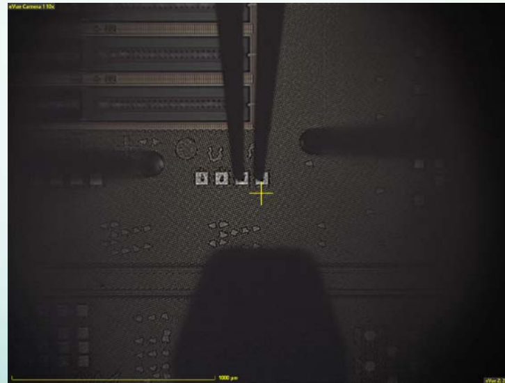
- Optical fibers and DC probe used for measurement - RF probe lifted and retracted since it is unused
