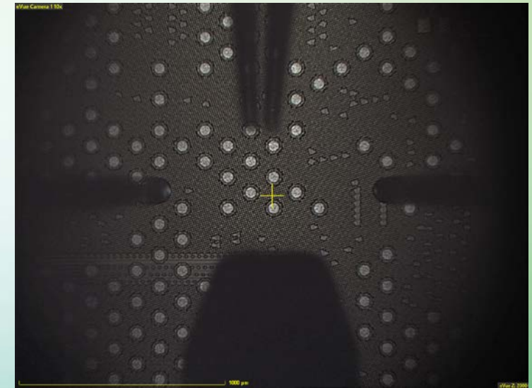
- Optical fibers used for measurement - DC and RF probe lifted and retracted since they are unused
