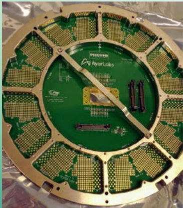
Traditional VLSI probe card -> no optical connectivity
