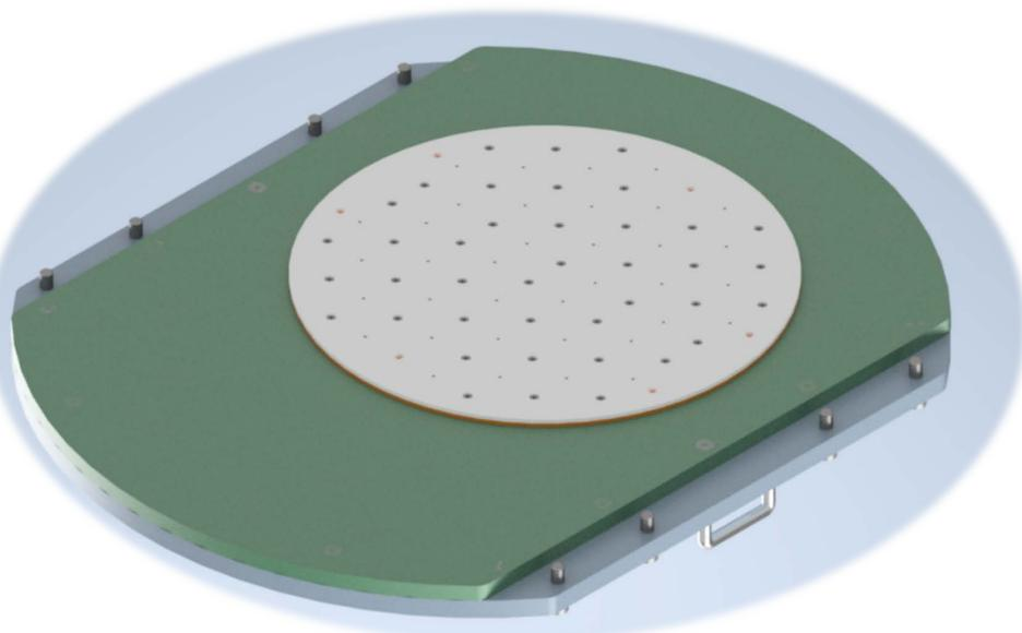
The aim of this project was to create a Probehead that could make full contact with a wafer in a single touchdown, 1118 probes over 86 sites.
