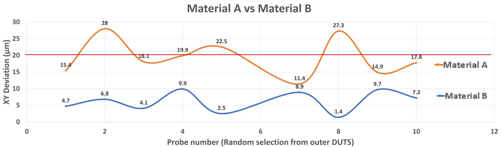
Here we can see a marked decrease in deviation between material A and material B. Any points above the red line are out of specification. Each deviation is measured in a direct line from the center of the designed XY to the center of the measured XY coordinates.
