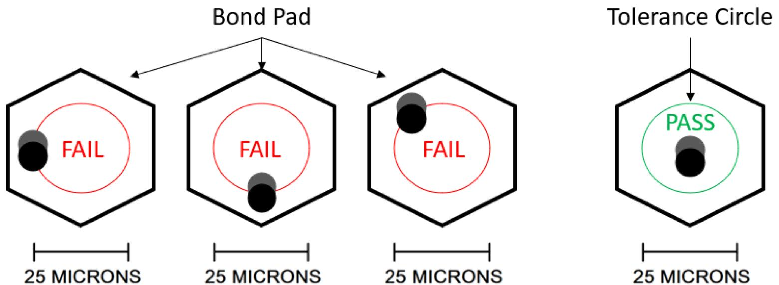
To verify this, we used an optical measurement tool to plot the final position of the pin tips against the specified XY coordinates. The figure below is an overlay of one of the outer sites – this shows the designed co-ordinate vs. tested position of the pin tip. You can clearly see a 28 $\mu\text{m}$  shift between the designed XY coordinates and the measured coordinates.
