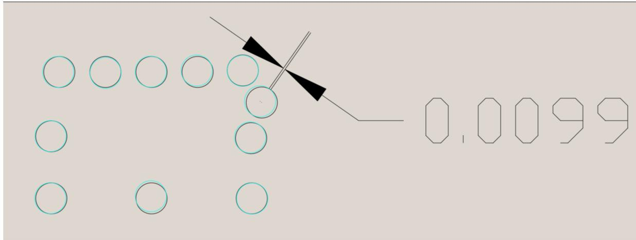
This shows the site with the highest deviation from the specified coordinates, at 9.9 microns movement.
