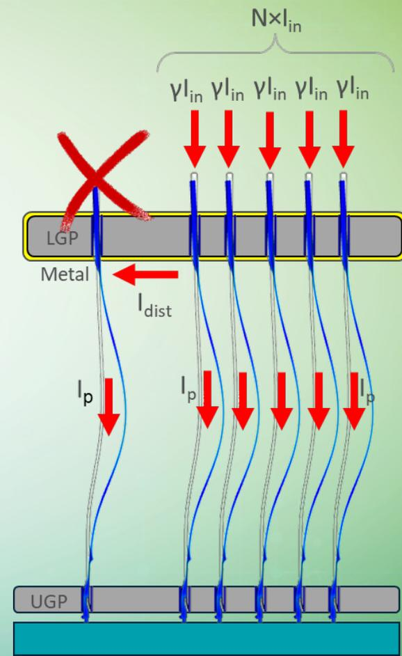
Poor contact or disconnect
