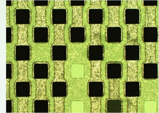
Metallization 2-Probe Circuit
