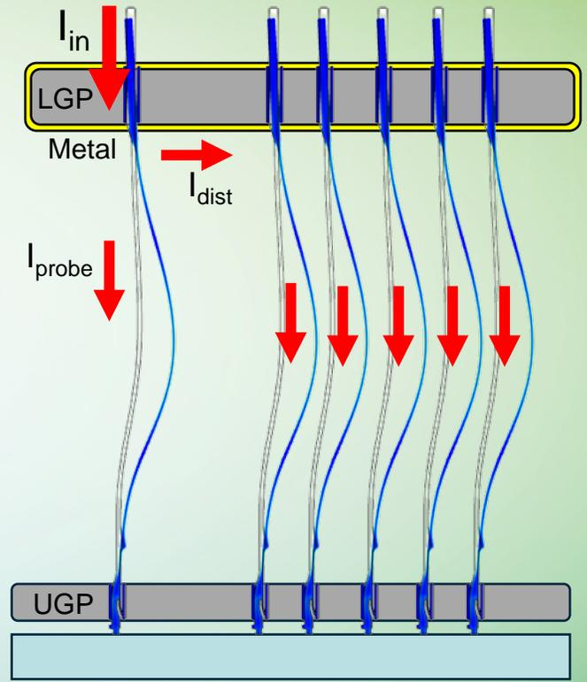
$$R_{dist} = \left( \sum_{n=1}^N \frac{1}{r_c + r_{tr(n)} + r_b} \right)^{-1}$$
