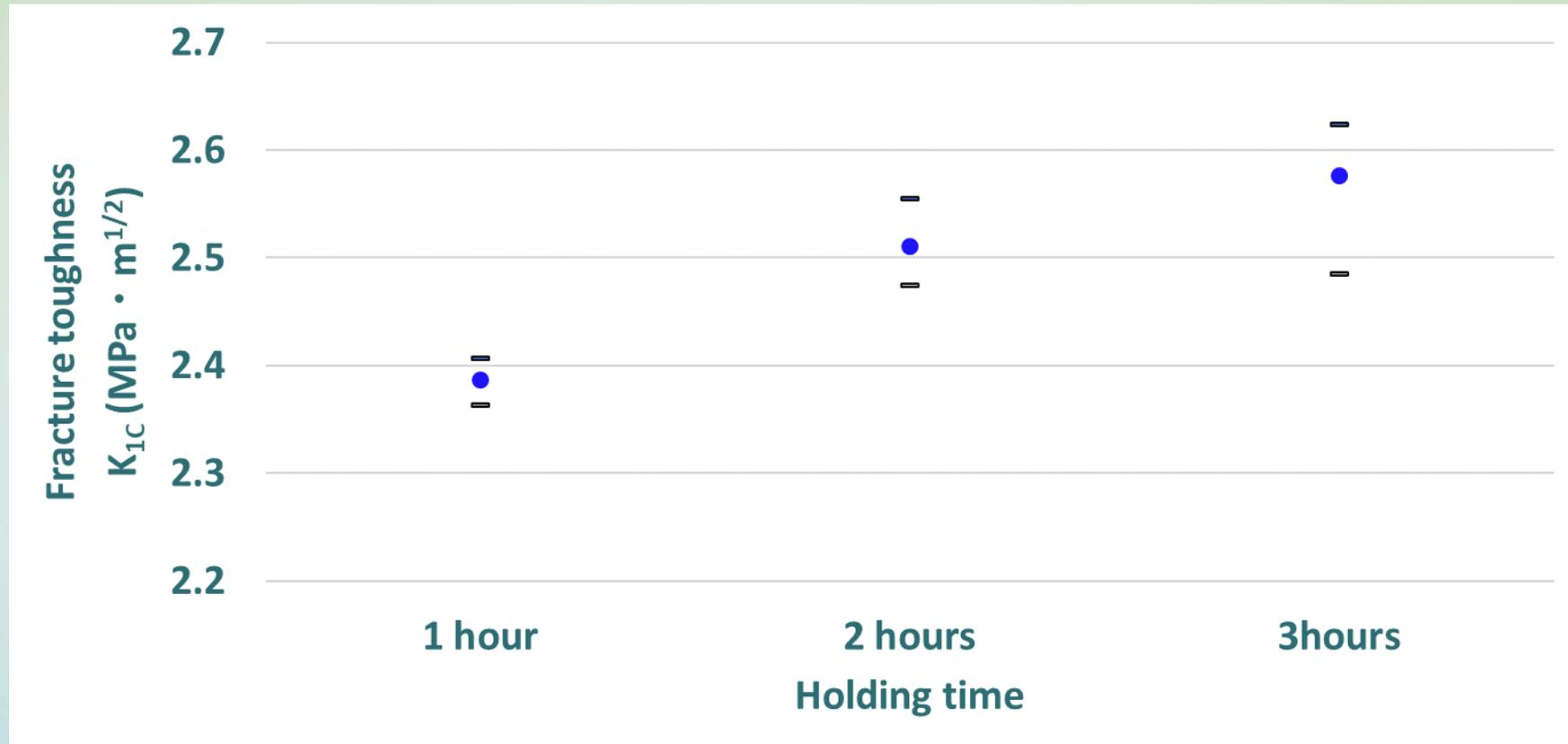
We believe that the improved fracture toughness is due to the anorthite precipitated in the glass region.
