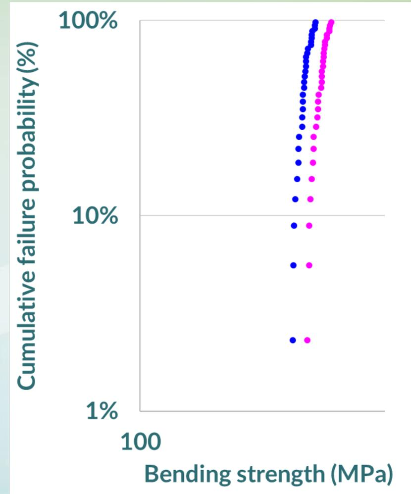
As the average particle size of the glass powders decreases, the void area decreases and the bending strength increases.
