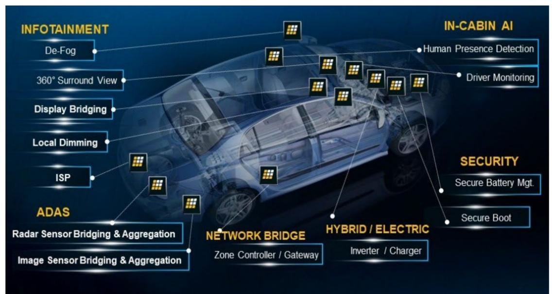
automobile contains at least, at least 10-12 FPGA's to control all of the systems with at least 5-7 more processors connecting all of the systems together. This doesn't even include all of the standard electronics for tire pressure sensors, backup camera, mems sensors, and crash avoidance.
