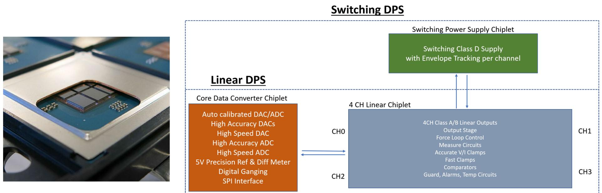
Additionally, depending on how the market changes, different blocks can be changed to support more channels, more voltage, larger accuracy, better efficiency, or any unforeseen requirements that may arise.
