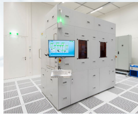
Advanced Resist Processing EVG®150 Series
