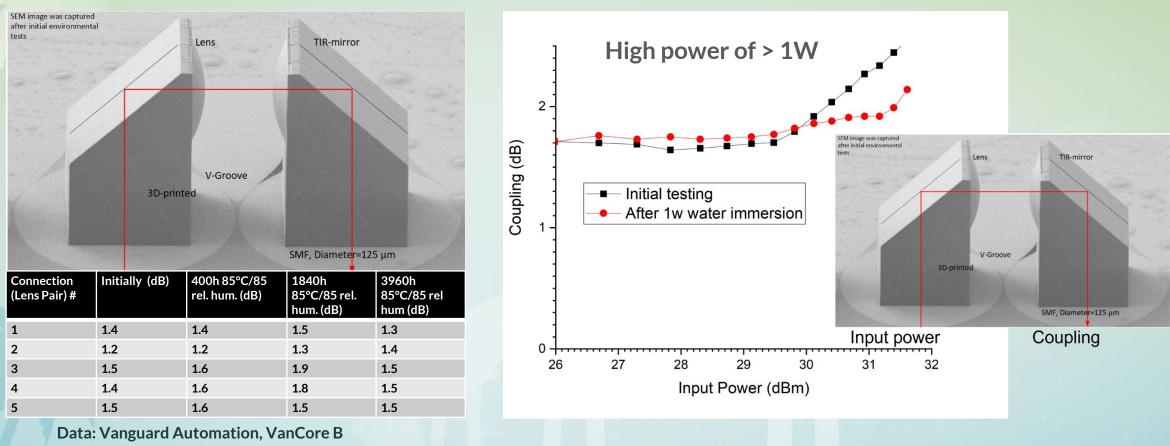
85°C, 85 % rel. hum.; -40/85°C cycle; 10 cycles from -4K to RT, N2 immersion
