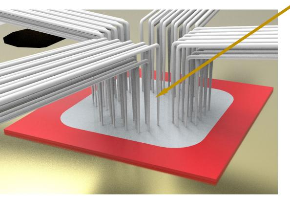
*Physical constraints of cantilever probe cards*
