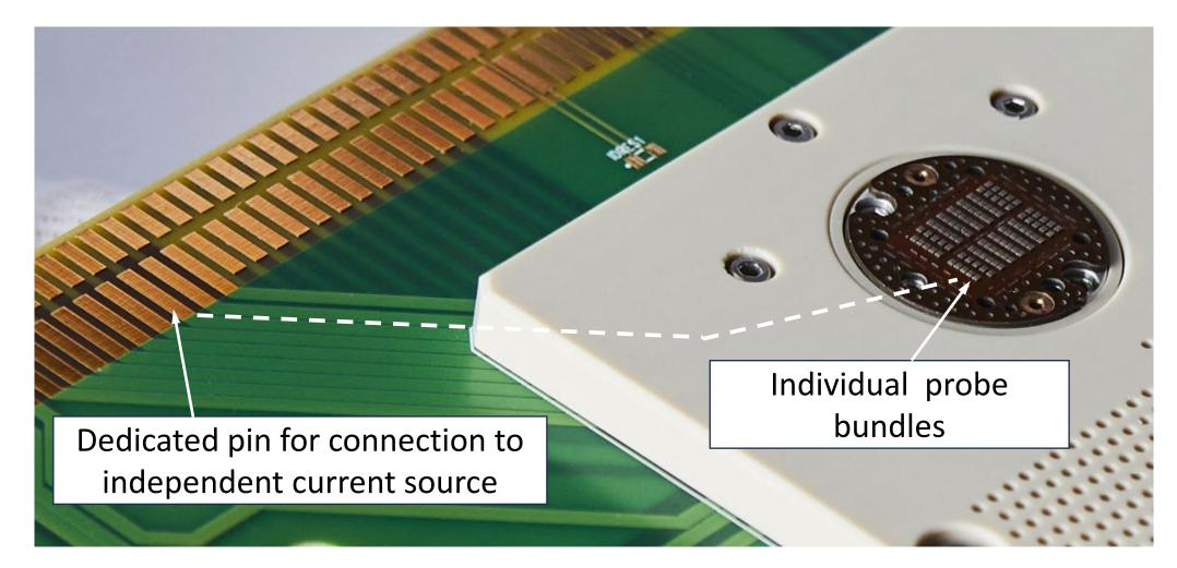
Independent current source connected to individual probe bundle
