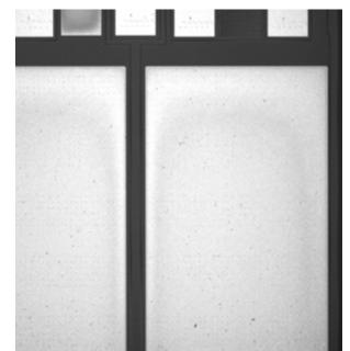
test. Once test is finished, the metal gets solid again and is soldered to probe tip. Parts of **metallization** (nuggets) are then **pulled out** when de-contacting.
