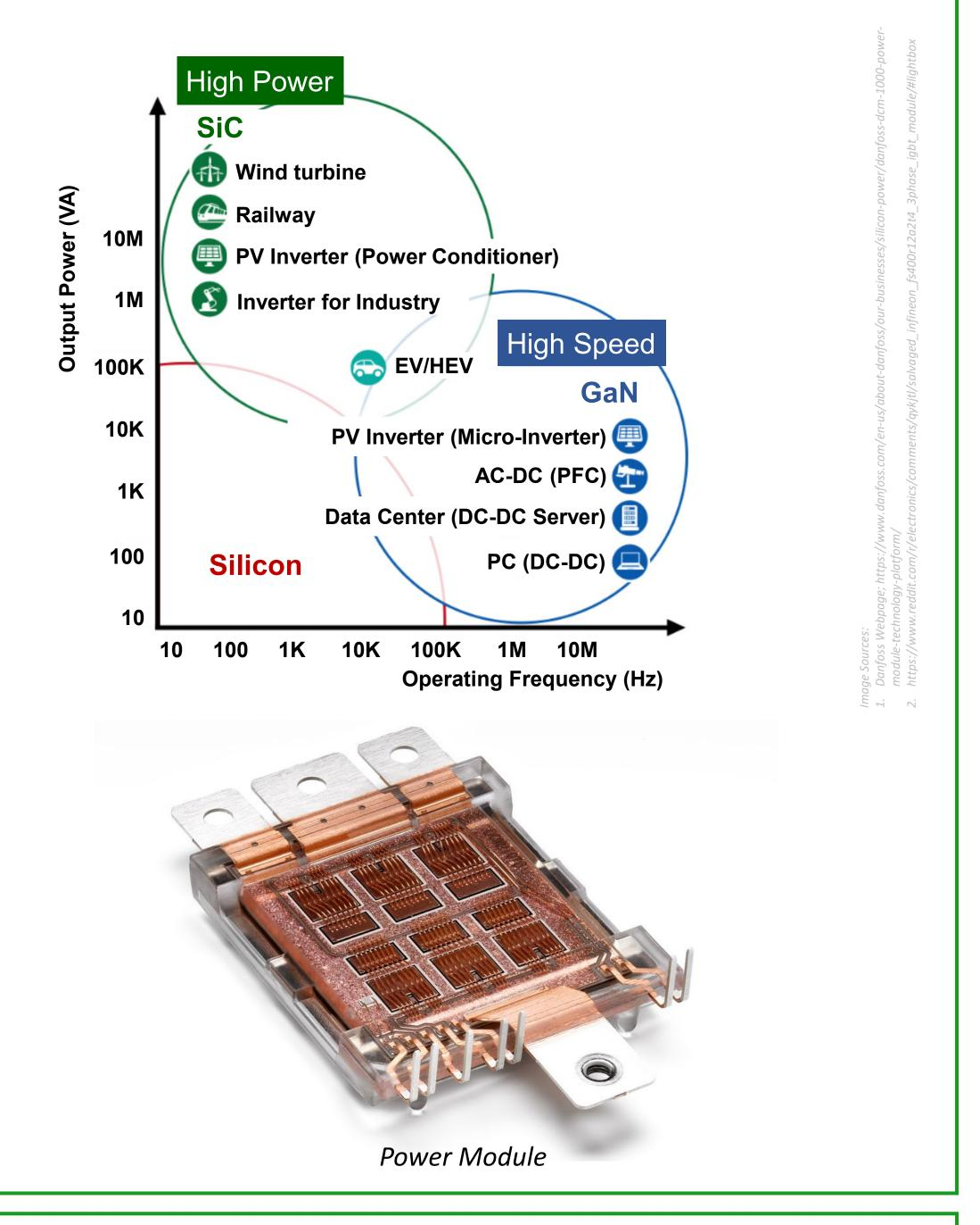
SiC devices have best efficiency at medium switching frequency and very high voltage/power.
