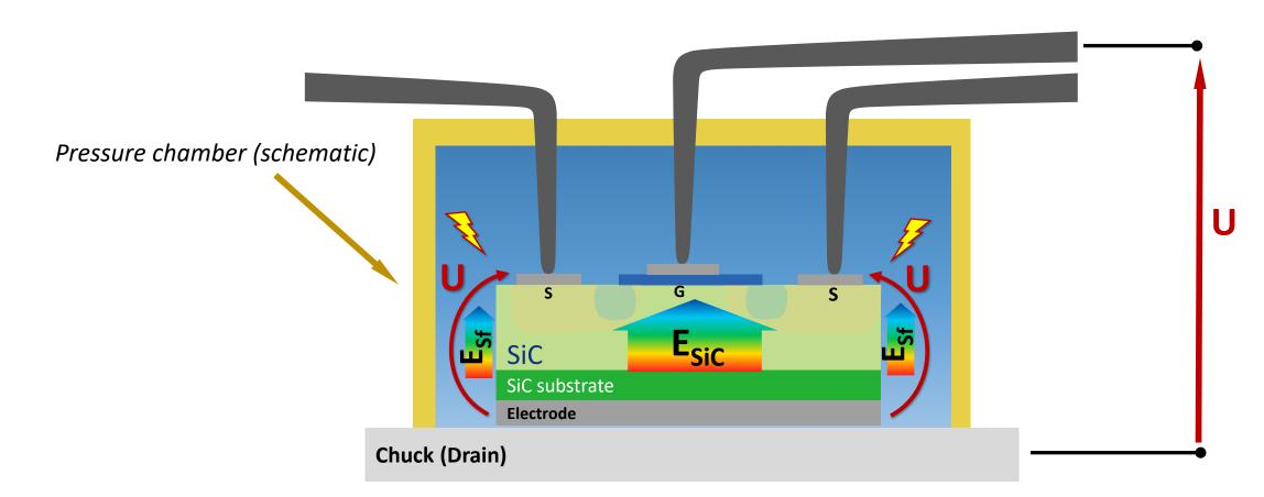
High voltage KGD test with arcing suppression
