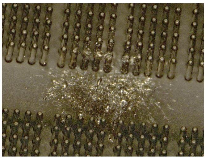
Liquid metal splashed on the probe head
