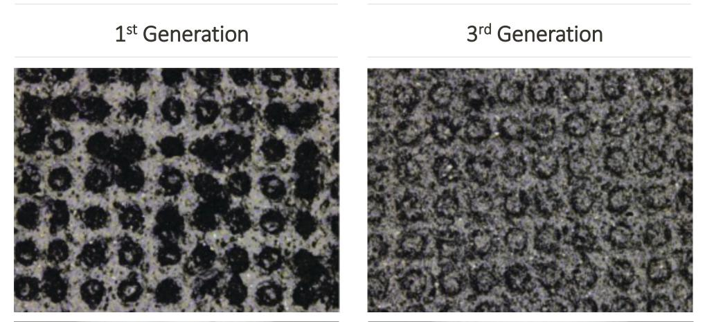
• Material surface imaged using a combination of optical and laser confocal microscopy to measure depth of damage.
