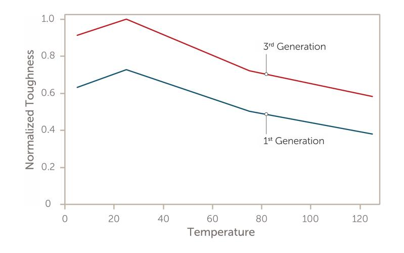
• 3<sup>rd</sup> generation materials have higher toughness across all temperatures and exhibit lower material damage at high temperatures.
